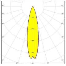
Dimensions: 109.7 mm x 109.7 mm Height: 17.10 mm ~24° medium beam
