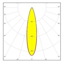
Dimensions: 9.9 mm x 9.9 mm Height: 7.50 mm ~25° diffused beam and holder with location pins
