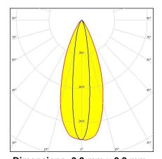
Dimensions: 9.9 mm x 9.9 mm Height: 7.50 mm ~40° x 20° oval beam and holder with location pins
