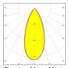
Dimensions: 9.9 mm x 9.9 mm Height: 7.50 mm ~50° wide beam. Clip fastening for
