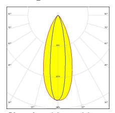
Dimensions: 9.9 mm x 9.9 mm Height: 7.50 mm ~40° x 20° oval beam. Clip fastening for 0.8 mm thick PCB.
