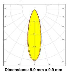
Height: 7.50 mm ~25° diffused beam. Clip fastening for 1.6 mm thick PCB
