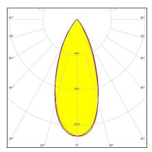
Dimensions: 9.9 mm x 9.9 mm Height: 7.50 mm ~50° wide beam and holder with location pins
