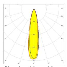
Dimensions: 9.9 mm x 9.9 mm Height: 7.50 mm ~19° real spot beam. Clip fastening
