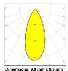
Height: 7.50 mm ~50° wide beam. Clip fastening for 1.6 mm thick PCB
