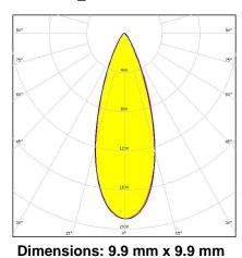
**Height: 7.50 mm**~30° medium beam. Clip fastening for 1.6 mm thick PCB.
