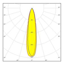
Dimensions: 9.9 mm x 9.9 mm Height: 7.50 mm ~19° spot beam. Clip fastening for 0.8 mm thick PCB.
