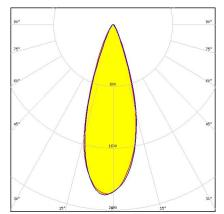
Dimensions: 10.0 mm x 10.0 mm Height: 6.80 mm ~35° wide beam. 6.8 mm high variant with location pin installation.
