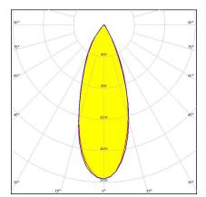
Dimensions: 9.9 mm x 9.9 mm Height: 6.80 mm ~35° wide beam optimized for CREE
