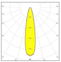
Dimensions: 9.9 mm x 9.9 mm Height: 6.80 mm ~19° spot beam. 6.8 mm high variant
