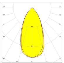
Dimensions: 9.9 mm x 9.9 mm Height: 7.00 mm ~45° wide beam. 7.0 mm high variant with location pin installation.
