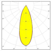
Dimensions: 9.9 mm x 9.9 mm Height: 6.80 mm ~35° wide beam. 6.8 mm high variant with location pin installation.
