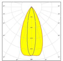
Dimensions: 10.0 mm x 10.0 mm Height: 6.81 mm ~45° x 20° oval beam. 7.13 mm high variant with location pin installation.
