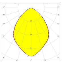
Dimensions: 9.9 mm x 9.9 mm Height: 7.00 mm ~80° wide beam optimized for CREE
