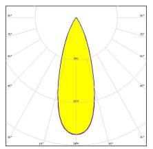
Dimensions: 9.9 mm x 9.9 mm Height: 6.60 mm ~20° medium beam optimized for LUXEON Rebel. 6.6 mm high variant with location pin installation.
