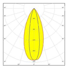
Dimensions: 10.0 mm x 10.0 mm Height: 6.81 mm ~45° x 20° oval beam optimized for CREE XP-E. 7.13 mm high variant with
