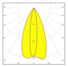
**Dimensions: 9.9 mm x 9.9 mm Height: 6.80 mm** ~45° x 20° oval beam optimized for CREE XP-E. 6.8 mm high variant with clip installation.
