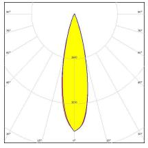
**Dimensions: 16.1 mm x 16.1 mm Height: 10.00 mm** ~25° medium beam. Assembly with holder, installation tape and pins.
