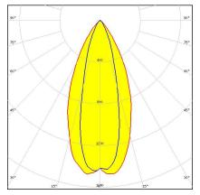
**Dimensions: 16.1 mm x 16.1 mm Height: 10.00 mm** ~45° + 15° oval beam. Assembly with holder, installation tape and pins.
