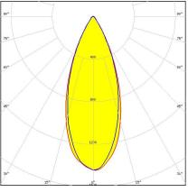
Dimensions: 16.1 mm x 16.1 mm Height: 10.00 mm ~36° wide beam. Assembly with holder, installation tape and pins
