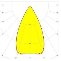
Dimensions: 16.1 mm x 16.1 mm Height: 10.00 mm ~55° wide beam. Assembly with holder, installation tape and pins. White version.
