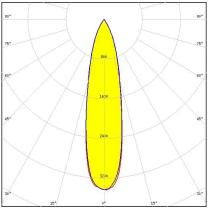
Dimensions: 110.0 mm x 110.0 mm Height: 65.00 mm ~24° medium beam
