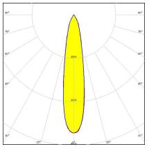
Dimensions: 110.0 mm x 110.0 mm Height: 65.00 mm ~15° spot beam
