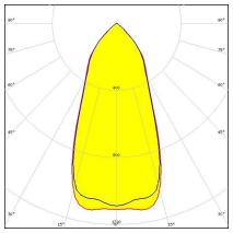
Dimensions: 45.0 mm x 45.0 mm Height: 21.10 mm ~40° wide beam. Assembly with installation tape.
