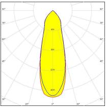
Dimensions: 45.0 mm x 45.0 mm Height: 21.10 mm ~30° medium beam. Assembly with installation tape.
