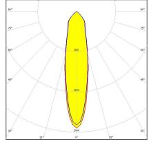
Dimensions: 45.0 mm x 45.0 mm Height: 20.10 mm ~25° spot beam. Assembly with installation tape.
