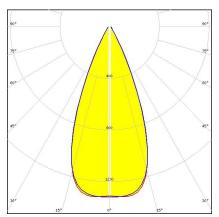
Dimensions: 50.0 mm x 50.0 mm Height: 15.30 mm ~20° medium round beam Dimensions: 50.0 mm x 50.0 mm Height: 15.60 mm ~20° medium beam
