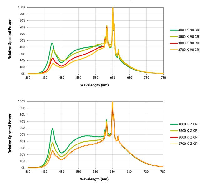
The following graphs are the result of a series of pulsed measurements at 1400 mA and T<sub>1</sub> = 85 °C.
