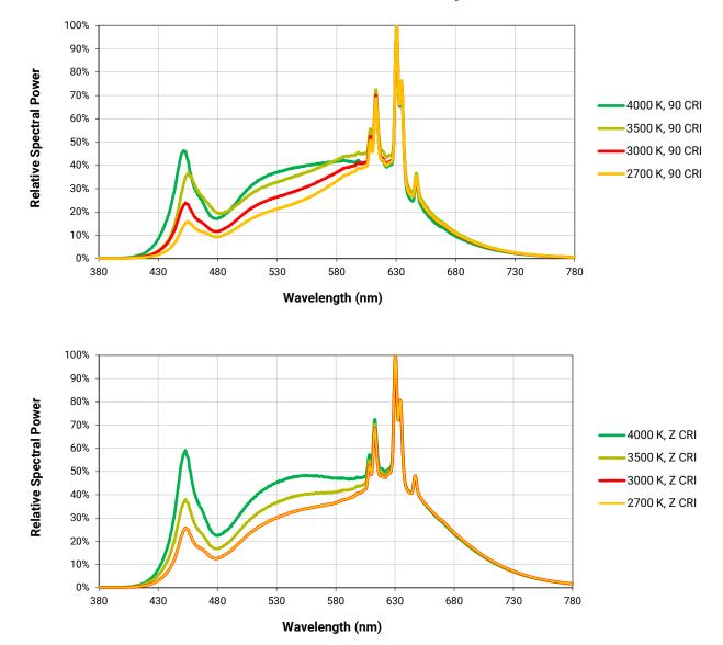
The following graphs are the result of a series of pulsed measurements at 360 mA and T<sub>1</sub> = 85 °C.
